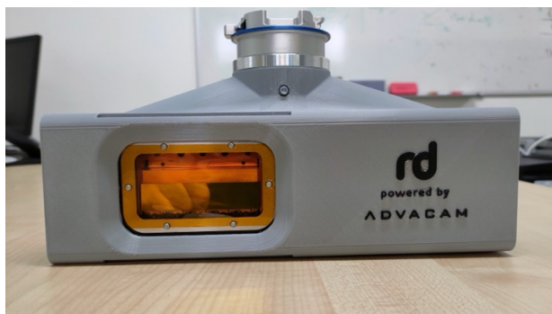
Obr. 2 Detektor WidePIX 1x5 Si PoE
