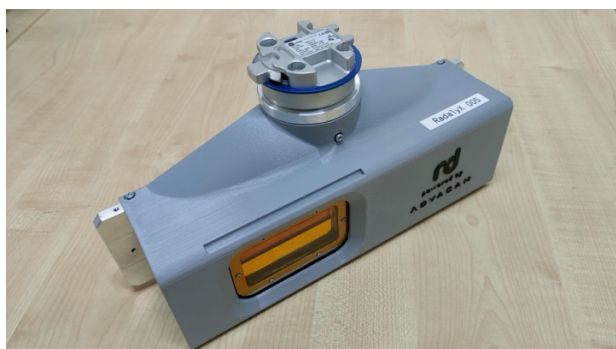
Obr. 2 Detektor WidePIX 1x5 Si PoE
